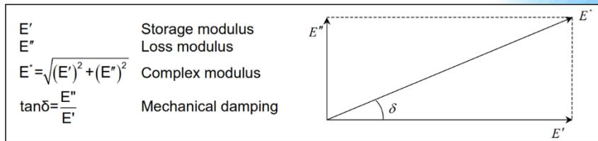
spring – quick to respond and returning nearly all the energy (not absorbing or dampening energy). The characteristics of the rubber recipe are adjusted using various polymers, fillers, plasticizers and other ingredients, specifically to adjust the ratio of elastic vs loss modulae. This allows Vernay Chemists to match the resulting rubber material properties specifically to the application and part criteria.
