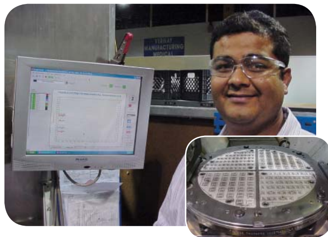
Ankur Maheshwari, program manager at Vernay Laboratories, stands next to the Priamus Heat closed-loop temperature controller that greatly reduced scrap in production of EPDM printer gaskets, each of which has 12 tiny O-rings. Inset: 112-cavity gasket compression mold.
