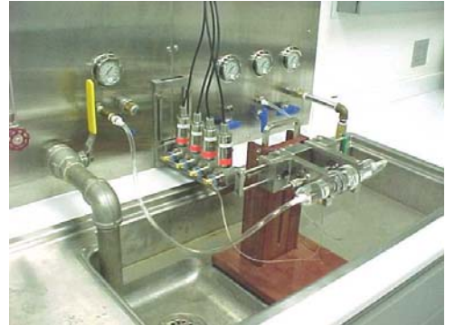
Water Test Bench with Fixture View
